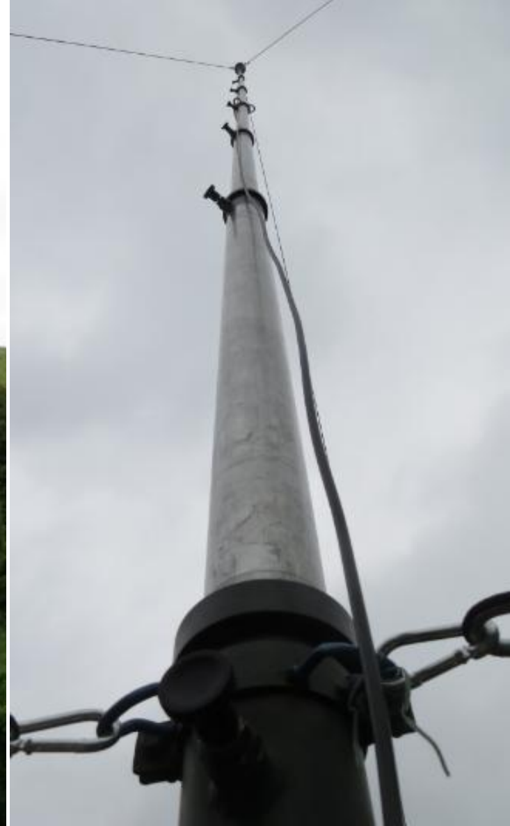
10m tall mobile pole with ultrasonic anemometer and data logger
