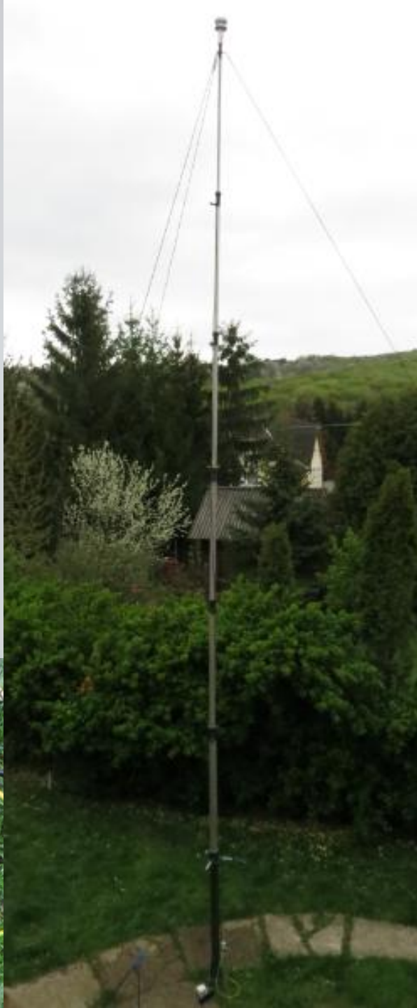
10m tall mobile pole with ultrasonic anemometer and data logger
